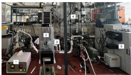
Fig. 1. Experimental setup (1- thermostat, 2- 1000 W lamp, 3- reactor, 4- mass flow controllers (MFC), 5- GC).
